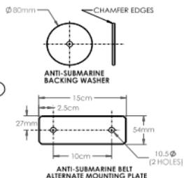
MOUNTING FASTENERS TO HAVE A MINIMUM TENSILE STRENGTH OF 150,000 PSI. AND BE CORROSION RESISTANT
