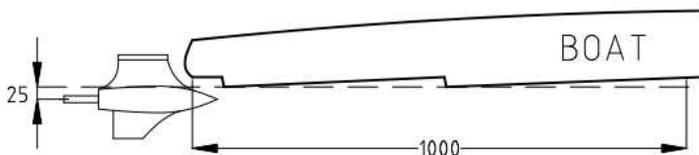
HYDROPLANE PROPELLER SHAFT HEIGHT MEASUREMENTS
