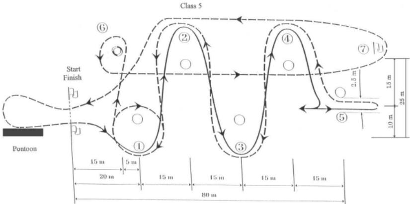
Departure - start line - along the course, turn around the gates 1, 2, 3, 4 from outside - by reversing to the gates 5 - again front motion, turn around the gates 4, 3, 2 from outside - quick detour of the gates 1 (the gates 1 are on the right side of the boat) - maneuver "man over-board" at buoy 6 - speed round: from inside gates 2 and 4, round buoy 7 and from outside gates 4 and 2 - finish line - return to pontoon - mooring
