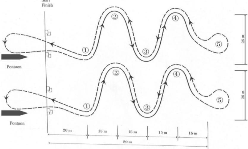
Departure - start line - along the course through the gates 1, 2, 3, 4, 5 - turning behind the gates 5 - again front motion through the gates 5, 4, 3, 2, 1 - finish line - return to pontoon - mooring
