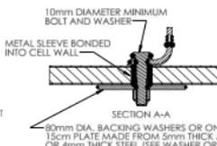
30mm DIA. BACKING WASHERS OR ONE 54mm x 15cm PLATE MADE FROM 5mm THICK ALUMINUM OR 4mm THICK STEEL (SEE WASHER OR PLATE SKETCHES)
