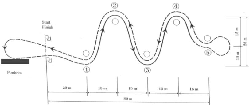
Departure - start line - along the course through the gates 1, 2, 3, 4, 5 - turning behind the gates 5 - again front motion through the gates 5, 4, 3, 2, 1 - finish line - return to pontoon - mooring
